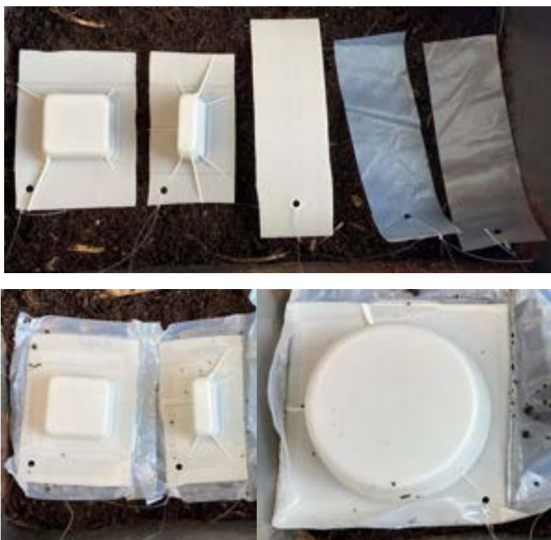
Figure 1. Summary of sample types utilized in lab composting trials - (top row, left to right) 1:5 scaled large thermoformed tray, 1:5 scaled medium thermoformed tray, 18-20 mil thermoforming sheet stock, 2 mil barrier-
