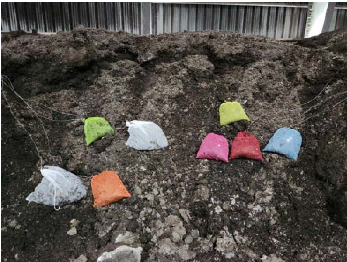
Figure 12. Distribution of samples in the compost pile during the second trial. From left to right, unmodified large bag (white), small tray with unmodified film lid (green), large tray with barrier-modified film lid (orange), barrier-modified large bag (white), small tray with barrier-modified film lid (pink), medium tray with barrier-modified film lid (yellow), large tray with unmodified film lid (red), medium tray with unmodified film lid (blue).
