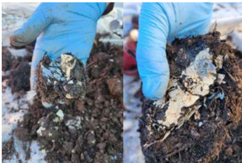
Figure 17. Example of degraded tray (small tray with unmodified film lid) with residual film stock on one surface face of the original tray (left), and localized area of diminished degradation for tray stock with film lid.
