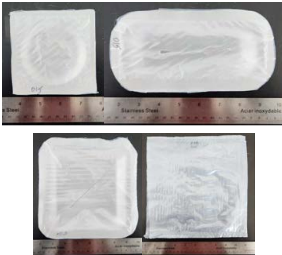
Figure 2. Compostable tray and bag prototypes produced using the pilot extrusion line. Displayed are small tray (top left), medium tray (top right), large tray (bottom left) and heat-sealed bag (bottom right).
