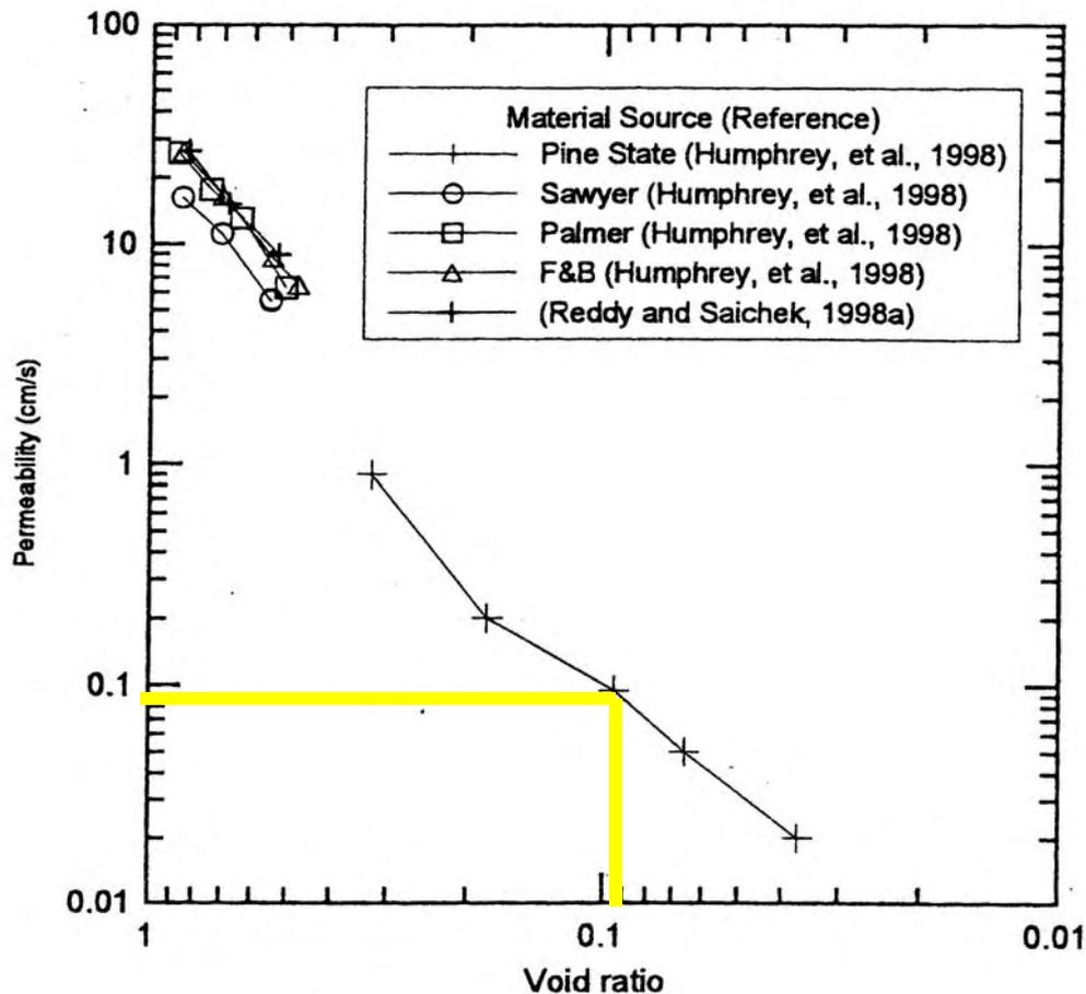
Material with a void ratio of 0.2 has a permeability of  $1 \times 10^{-1}$  cm/sec
