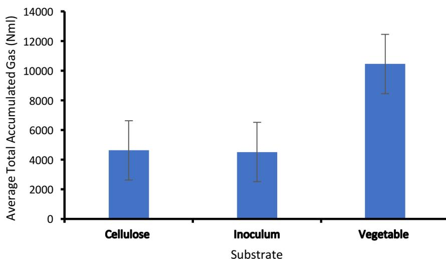
Figure 2. Average total biomethane gas levels recorded after a 30-day anaerobic digestion trial run at a mesophilic temperature of 38°C.
