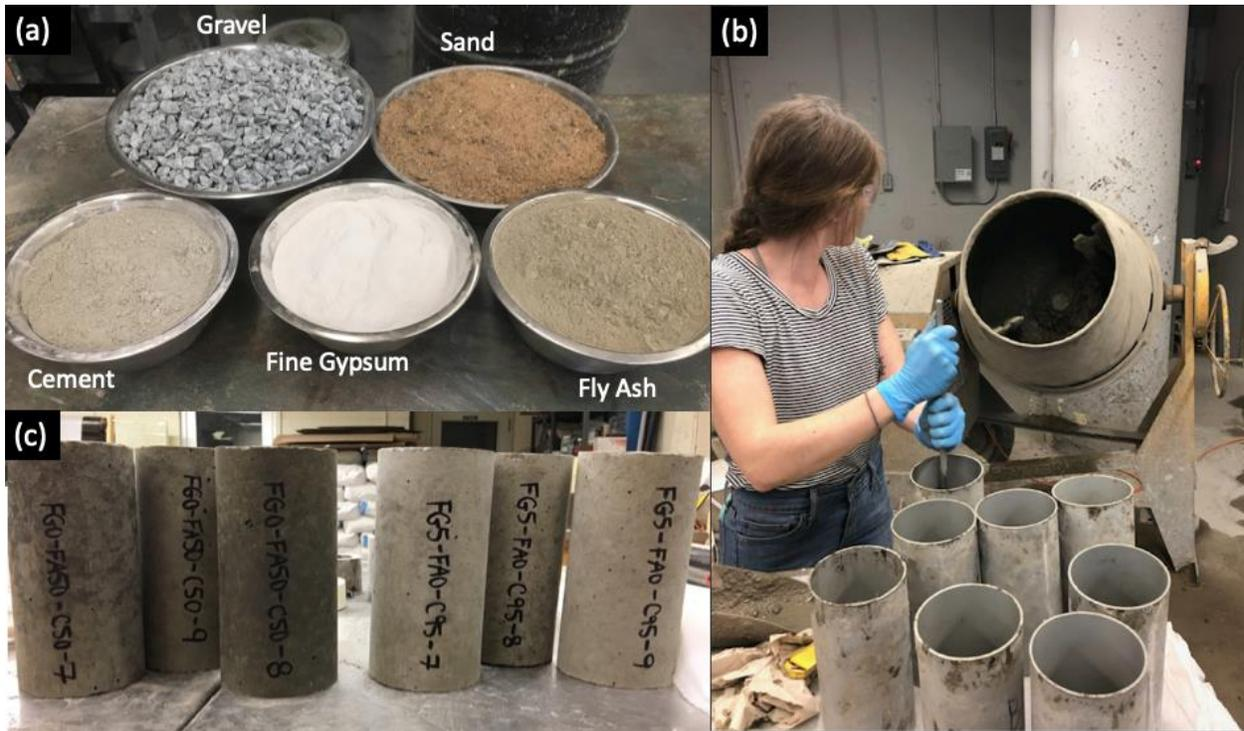
**Figure 4. Specimen preparation: (a) dry materials; (b) hand tamping; (c) comparison of specimens with and without fly ash**
