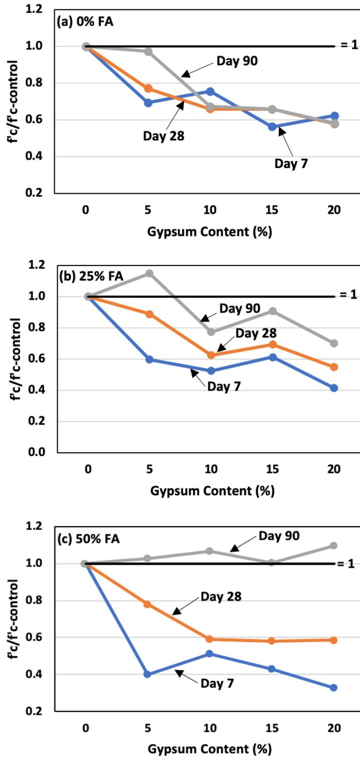
Figure 7. Compressive strength comparison to control mixes with varying gypsum content for (a) 0% FA; (b) 25% FA; (c) 50% FA
