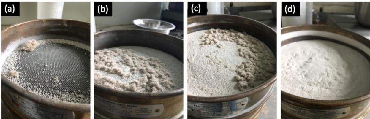
**Figure 2. Gypsum retained on sieves (a) No. 16; (b) No. 30; (c) No. 50; (d) No. 100**
