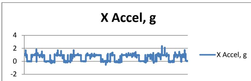
In the Excel graph, each switch from approximately +1 to 0 (X-axis) indicates a move from a lying position to standing position. Data shown is for a single cow (FS 7350 round 5) for 2 days. Analysis is on 300 cow records of 7 days each
