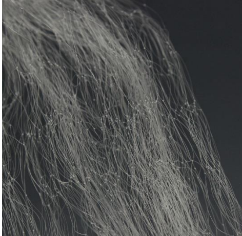
Figure 3. Monofilament polyethylene netting used in a gill net (SportsWorld.com).
