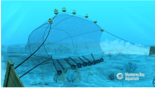
Figure 7. Depiction of the use of a bottom trawl net for fishing.
