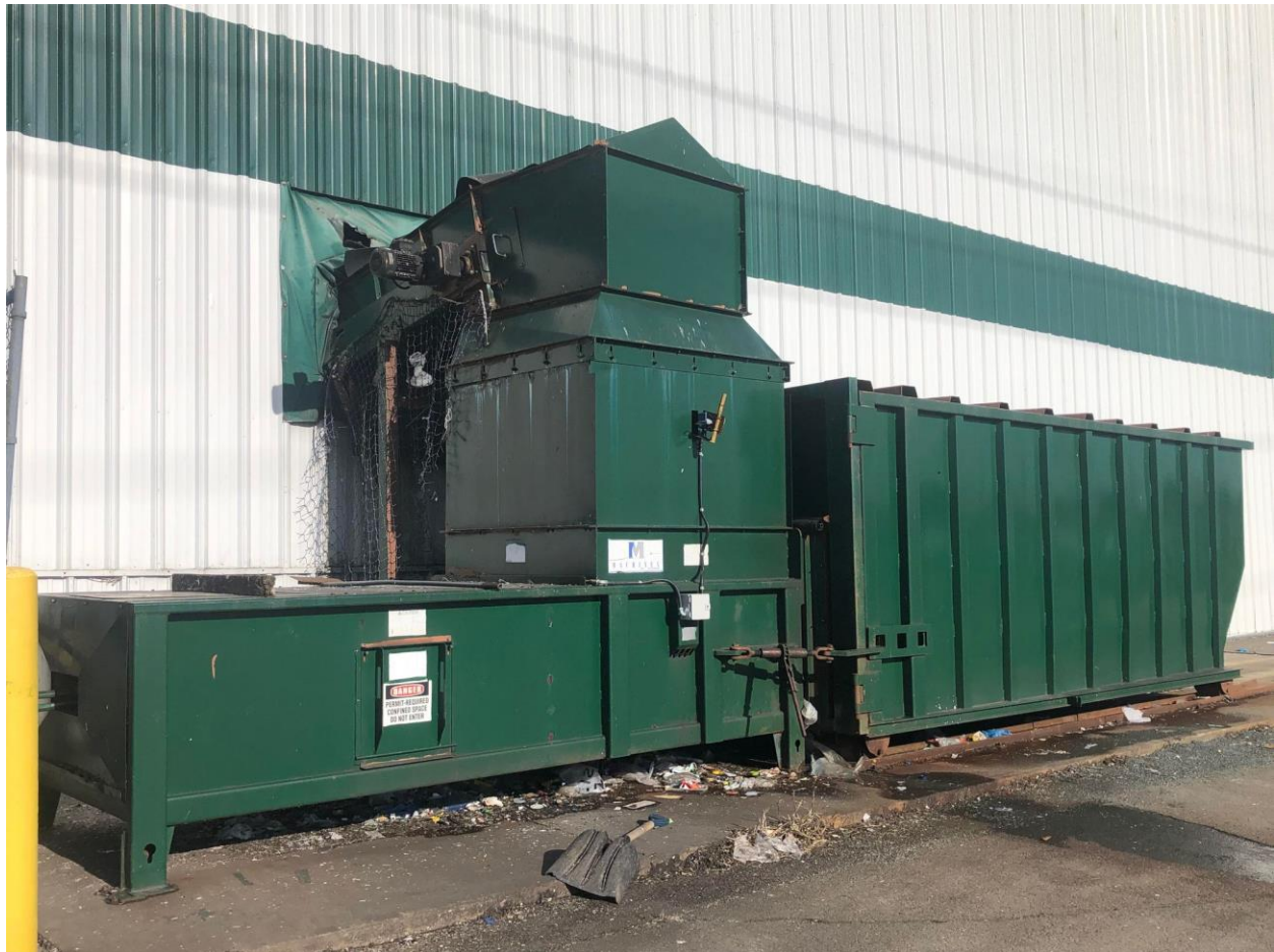
Figure 2 – Refurbished Exterior Compactor and Bin
