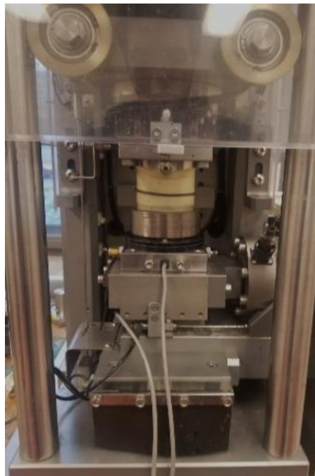
Figure 4.3: A DSS specimen mounted for testing
