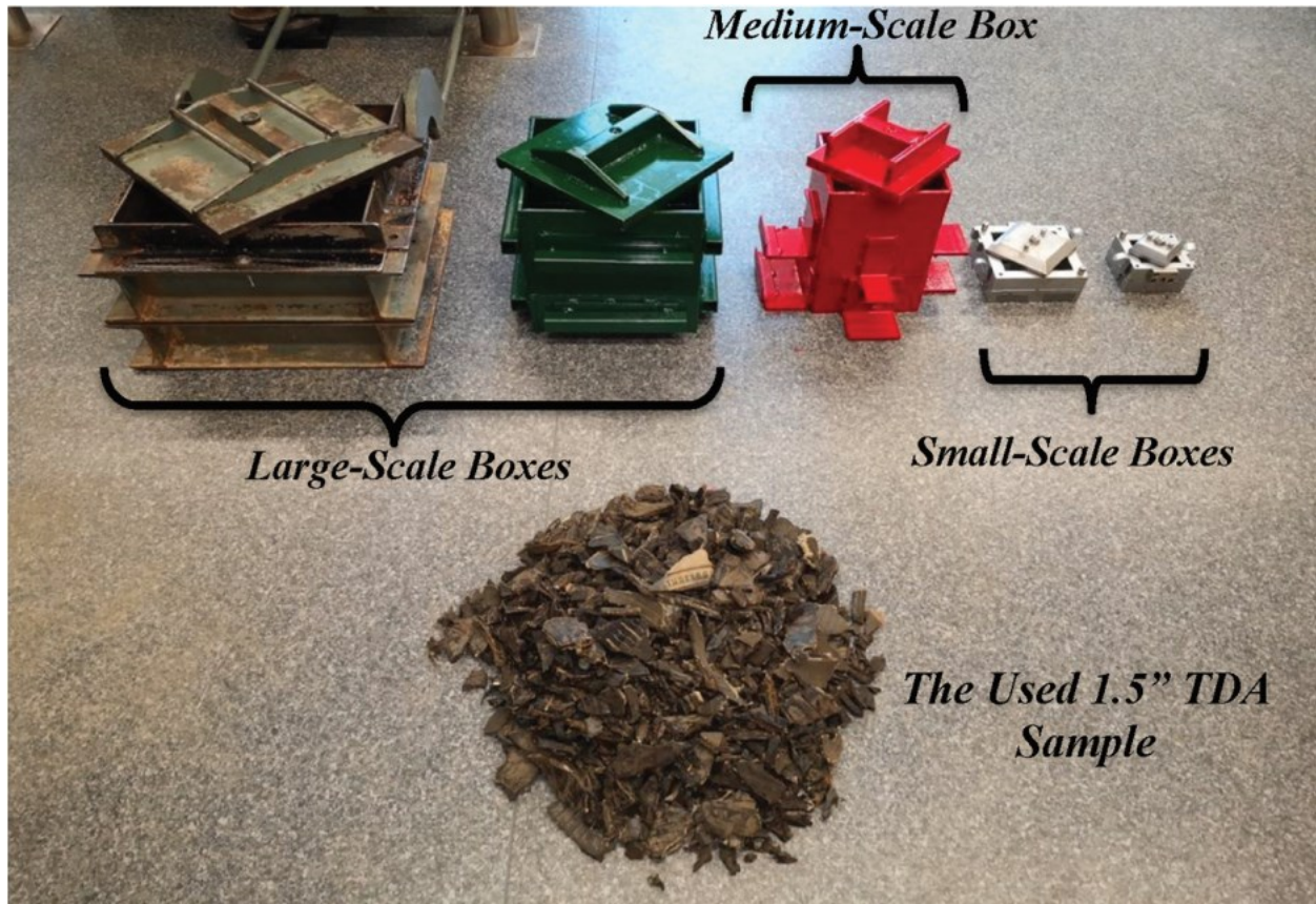
Figure 2.8: Shear boxes and tire-derived aggregate (TDA) sample used in the research.
