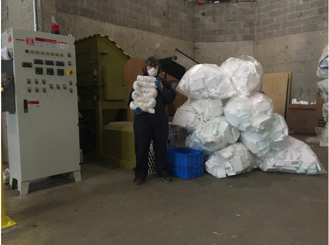
Figure D. 10 Amount of polystyrene densified into a single ingot
