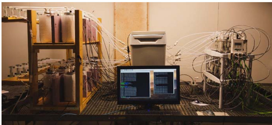
Fig. 21. Automated respirometry system at the University of Guelph. (Source: A. Dsouza, 2021)
