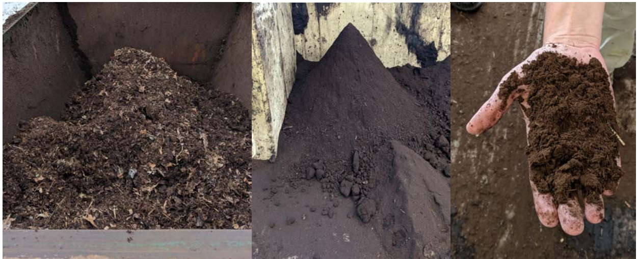
Fig. 4. Raw organic waste feedstock in HotRot 1811 hopper (left), processed material exiting the composting system (centre), and final material used for plant production experiments (right).
