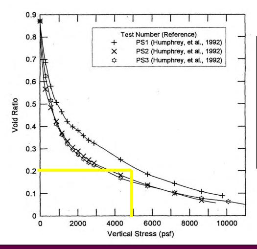
Void ratio of 0.2 limits vertical stress to 5,000 psf or about 67 feet of solid waste
