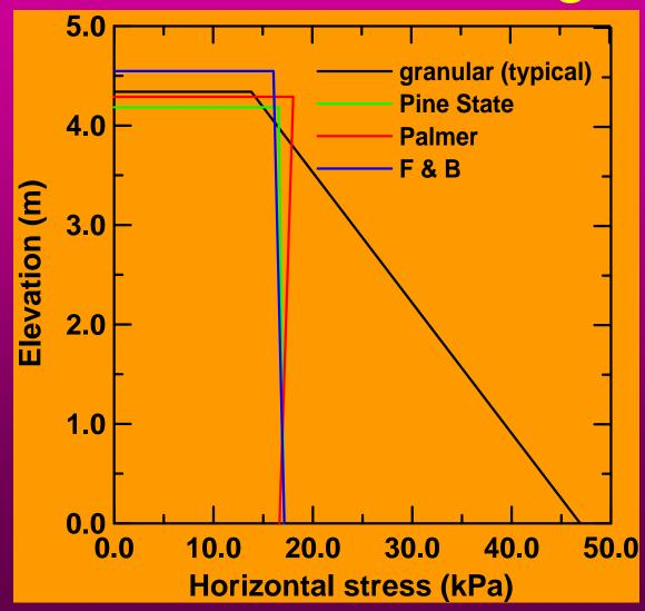
Rotating wall away from backfill
