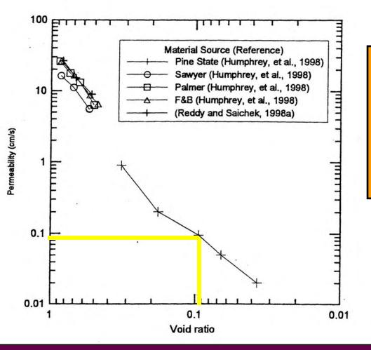
Material with a void ratio of 0.2 has a permeability of 1x1<sup>-1</sup> cm/sec
