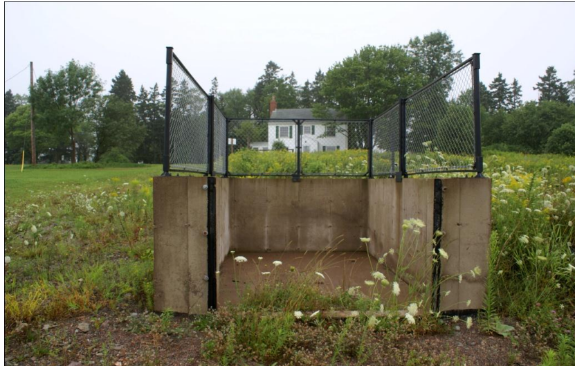
Figure 6. Picture of Lysimeter Cell used located at the BEEC research site, Bible Hill, NS.
