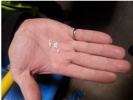
Figure 4. EPS beads after expansion due to pentane gas.
