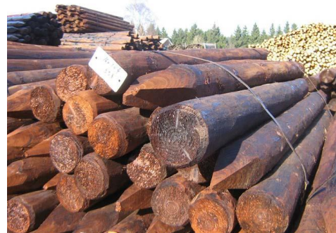
Figure 2.8 Creosote Treated Fence Posts
