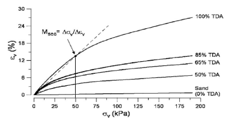
Fig. 8. Vertical strain  $(\varepsilon_v)$  versus stress  $(\sigma_v)$  for TDA specimens (tire chips) tested in the oedometer
