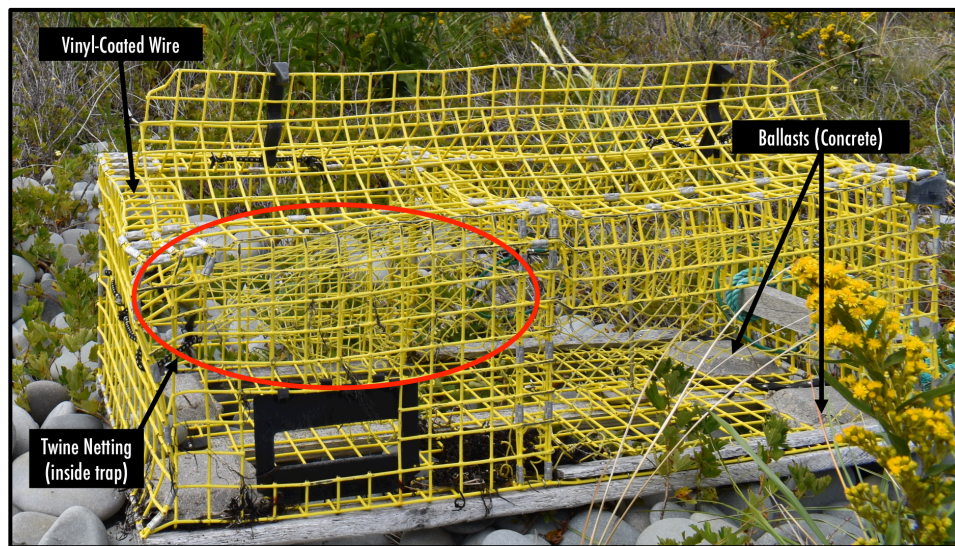
Figure 4. Diagram showing the parts of a wire lobster trap. Photo copyright Rachel A. Kendall.
